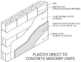
**CMU (Concrete Masonry Units)** make an excellent base for cement plaster. Raw CMU provides suction and a good key for cement, lath is not required. Bonding agents can be used to insure bond. Test areas are recommended. ½ to 5/8 inch thickness generally requires no lath over clean CMU walls. Cement plaster over 5/8 inch thickness, should have a lath applied.
