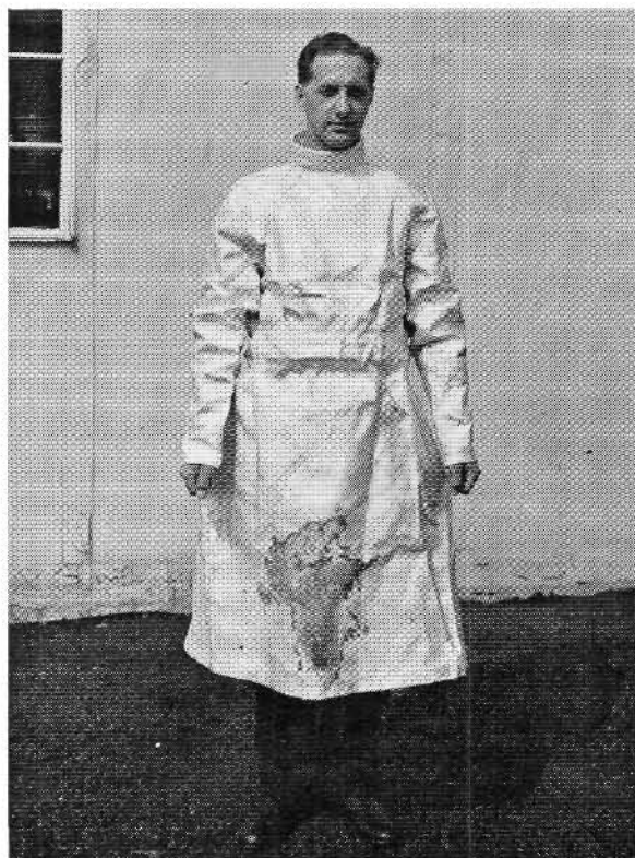
Fig. 7.—Coat damaged by splash of burning sodium
