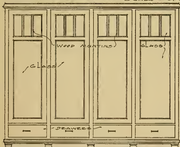
ELEVATION OF BOOK CASE - ELEVATION OF BUFFET SCALE 1/2" = 1'-0"
