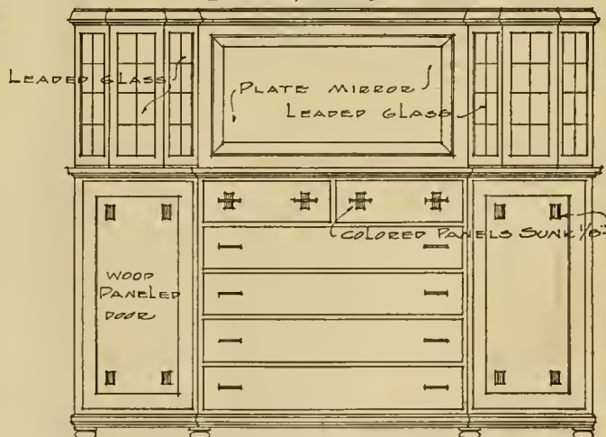
ELEVATION OF BOOK CASE - ELEVATION OF BUFFET SCALE 1/2" = 1'-0"
