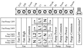
\*Note: Use the provided wire nut to connect all ground connections for power supply, fan, pump, purge pump and cooler cabinet.
