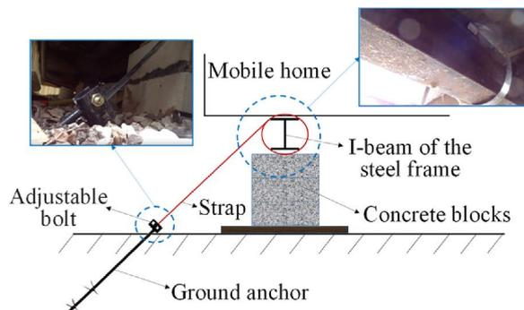
Fig. 1. Standard in-ground anchoring system for manufactured/mobile home.
