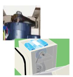
1 During shipping, the slack cable device may engage and need to be reset.
