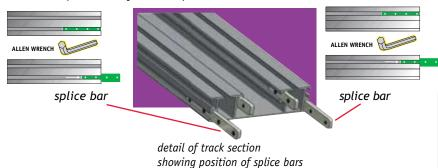
**9** Slide the upper track section onto the lower track section. Tighten the splice bar set screws to lock tracks together.
