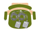
2 Remove the two screws from the back of the backrest. Use them to attach the backrest to the preferred height position on the seat back bar.
