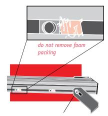
NOTE: attach a bracket on the bottom nut, but leave the nut second from the bottom unused – it will be used later.
