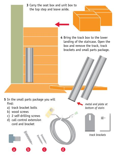
**6** Identify the bottom track section. It will have a *metal end plate* at one end. Lay the lower track section on the steps as shown in the picture above. **NOTE:** Top track section will be installed with the unit after installation of bottom and mid tracks. It requires 2 brackets.
