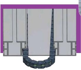
Note: Check every chain link. If unsnapped, the chain will not bend correctly.
