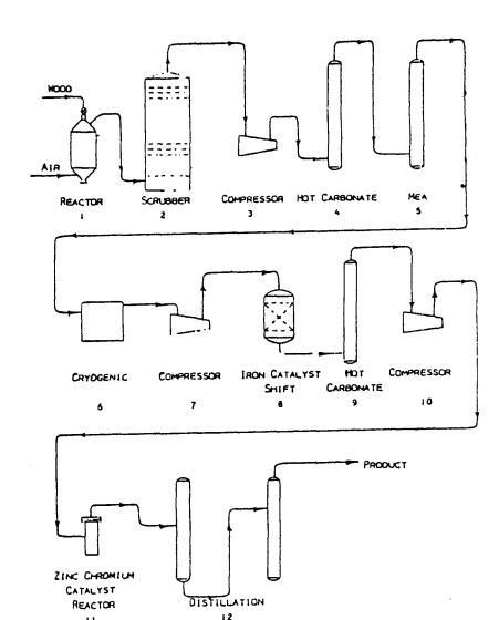
Figure 7.--Methanol synthesis from wood waste.
