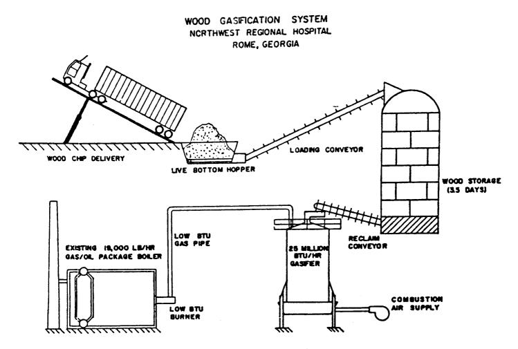
Figure 5.--Wood gasification system at Northwest Regional Hospital in Rome, Ga.
