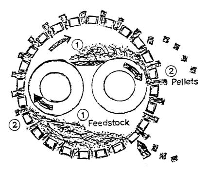
Figure 3. --Pelleting process.
