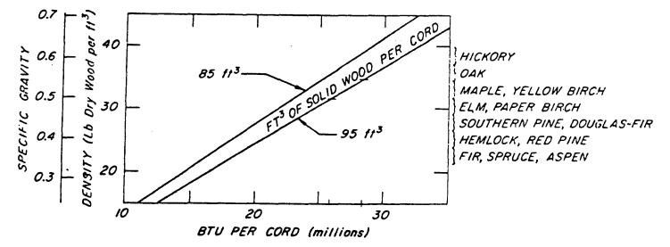
Figure 1.--Graph to estimate the higher heating value of a cord of wood knowing either species, specific gravity, or density. Higher heating value is defined as the theoretical amount of heat obtainable from 1 cord of wood containing no moisture. The actual heat obtainable will be about 60 percent of this estimate if air-dried wood is burned in a well-designed wood burner.
