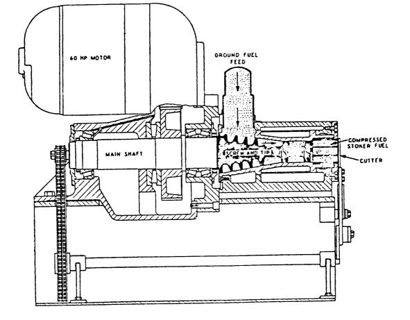
Figure 2. -- Pres-to-Log stoker-fuel machine.
