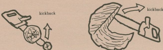
Figure 8. Kickback is a common cause of chainsaw injury to an operator. Hitting an object with the nose of the moving chain will throw hundreds of rapidly moving blades at you. Do not operate your saw beyond your capacity of experience. Ask your chainsaw dealer for the safety rules published by the Chain Saw Manufacturers Association.
