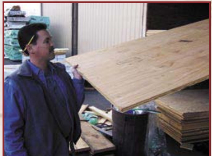
Figure Two: Inspecting plywood for fire-rating.
