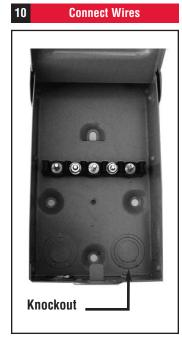
10. Remove the knock out in the lower right corner of the external connection box. From the rear of the connection box, feed wires & 4-pin plug into box. Slip the lock nut over wires and plug and tighten securely onto conduit coupling. Connect the black, red, and white wires to matching wires on threaded lugs and tighten securely. Fasten the green ground wire securely to the lug on the bottom of the box. The male end of the 4-pin plug is not connected at this time.
