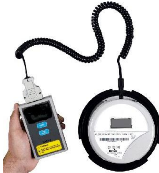
Figure 18: ZRO-C2A Resetter Connected to the CENTRON
