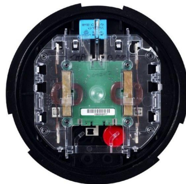
Figure 4: CENTRON 20 Amp Metrology
