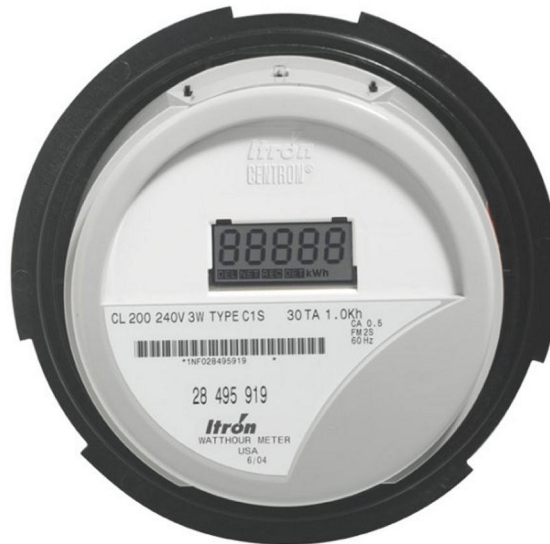
Figure 16: C1S LCD Personality Module
