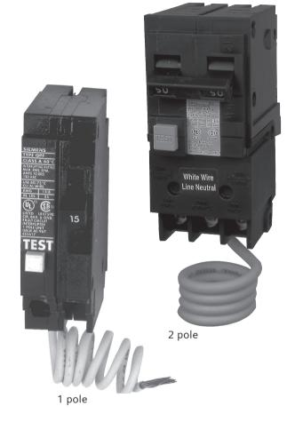
Siemens GFCI circuit breakers are UL Listed and CSA Certified as Class A devices. Current imbalances of 4-6 milliamps or more between load conductors will cause the ground fault sensor to trip the circuit breaker.
