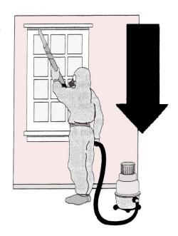
work towards the decon. Begin with ceilings or the top of the walls and work down, cleaning the floors last. Do every inch of the windows, especially the wells. Use the corner tool to clean where the floor meets the baseboard and all cracks in the floor boards. Use the brush tool for the walls. Move slowly and carefully to get all the dust.
