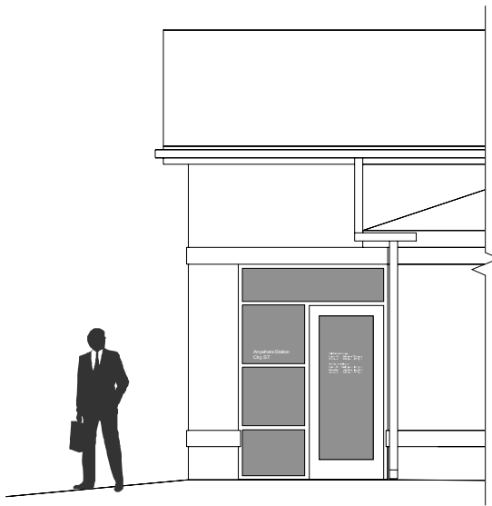
Exhibit 3-5n Typical elevation of entrance with vinyl placement for SSBD plans 40, 50, 65A, 80A, and 100A
