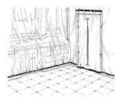
Step 1 – Use the plastic sheeting to isolate doorways and cover floor registers, vents, and other surfaces to prevent contamination from asbestos fibers.
