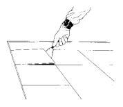
**Step 3** - Use a wide putty knife or flat floor scraper and gently pry up the tiles. Keep the tiles in *whole pieces*, <u>do not</u> break material on purpose, <u>do not</u> step on material, and <u>do not</u> drop material. Place the material on the ground in a non-work area or in separate containers to prevent breakage. Once the material has been removed, it may not be broken further.
