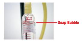
The soap bubble should be at the 100 ±5 ml mark. If it is not lubricate the pump and repeat Steps 1-8.
