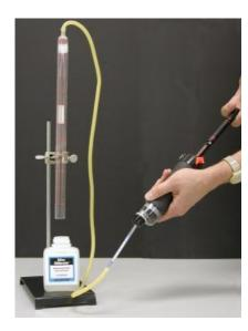
Take a full pump stroke and observe that the bubble has stopped moving (about 1 minute for a 120SD tube).
