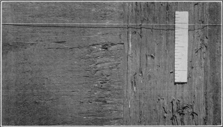
FIGURE 11.— Quarter-sawn red oak 2\frac{5}{32} inch thick, set in mastic.
