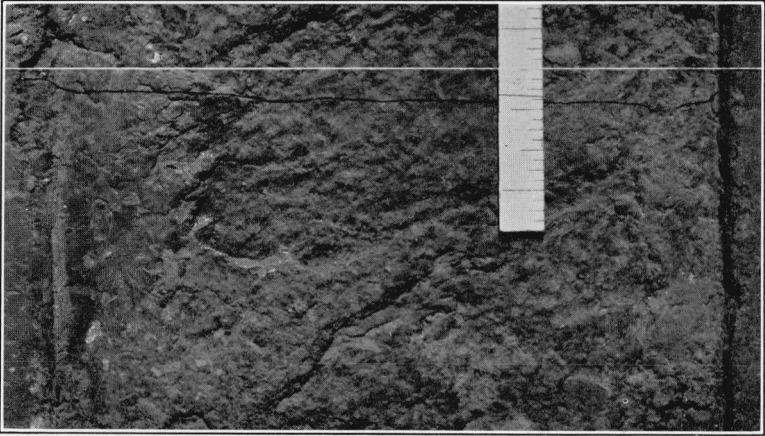
FIGURE 8.—Asphalt plank \frac{1}{2} inch thick.
