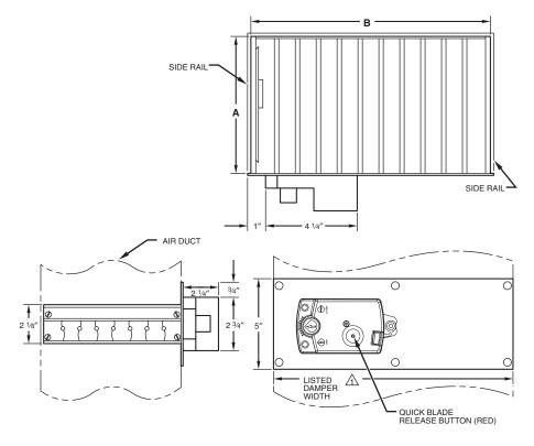
Fig. 2 – Bottom–Mount Damper Configuration
