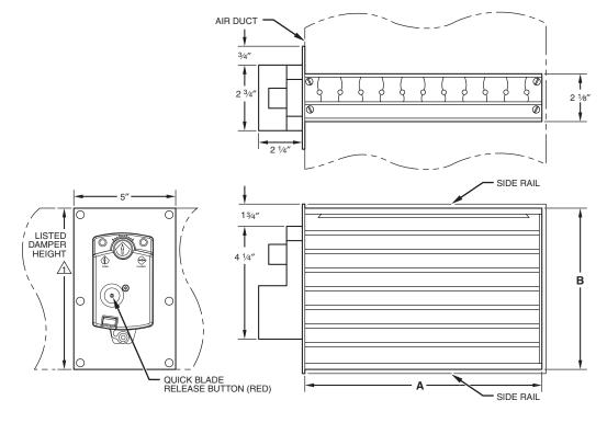
Fig. 1 – Side–Mount Damper Configuration
