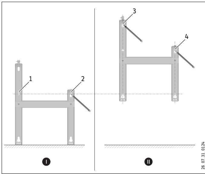
» Drill holes at all four markings. Secure the wall mounting bracket with suitable materials (screws, rawl plugs) depending on the type of wall. With the vertical slots, you can compensate for an offset fixing hole.
