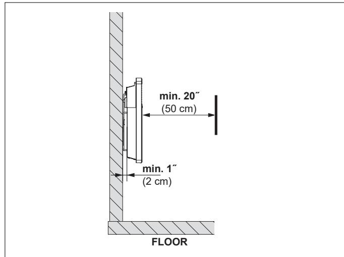
» The image above shows minimum allowed clearances between the installed appliance and any hard surfaces.
