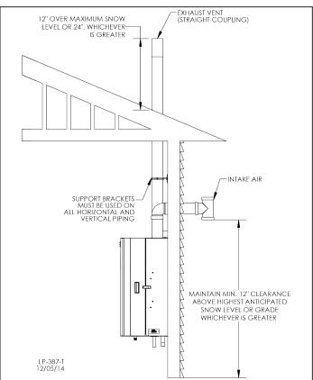
Figure 20 - Unbalanced Venting - Roof Exhaust and Sidewall Intake
