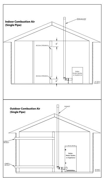
Figure 23 - Indoor and Outdoor Combustion Air - Single Pipe
