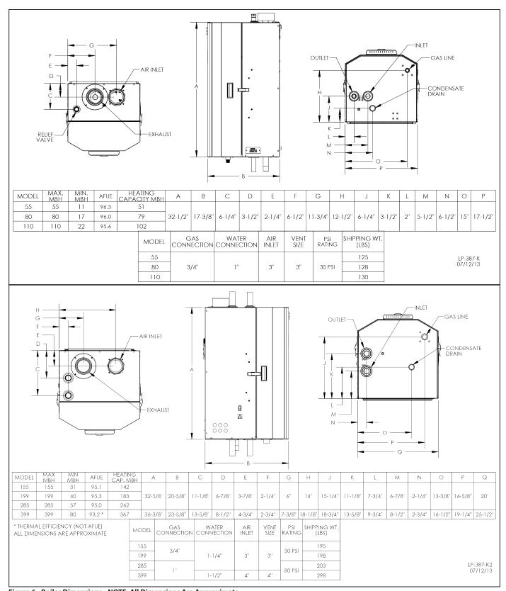
Figure 6 - Boiler Dimensions - NOTE: All Dimensions Are Approximate
