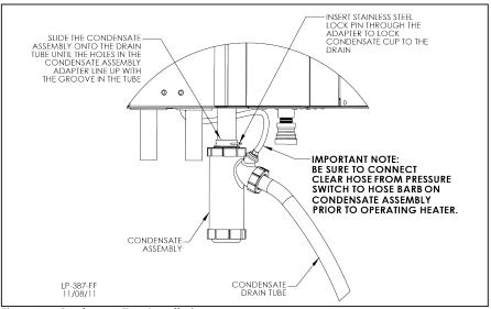
Figure 25 - Condensate Trap Installation
