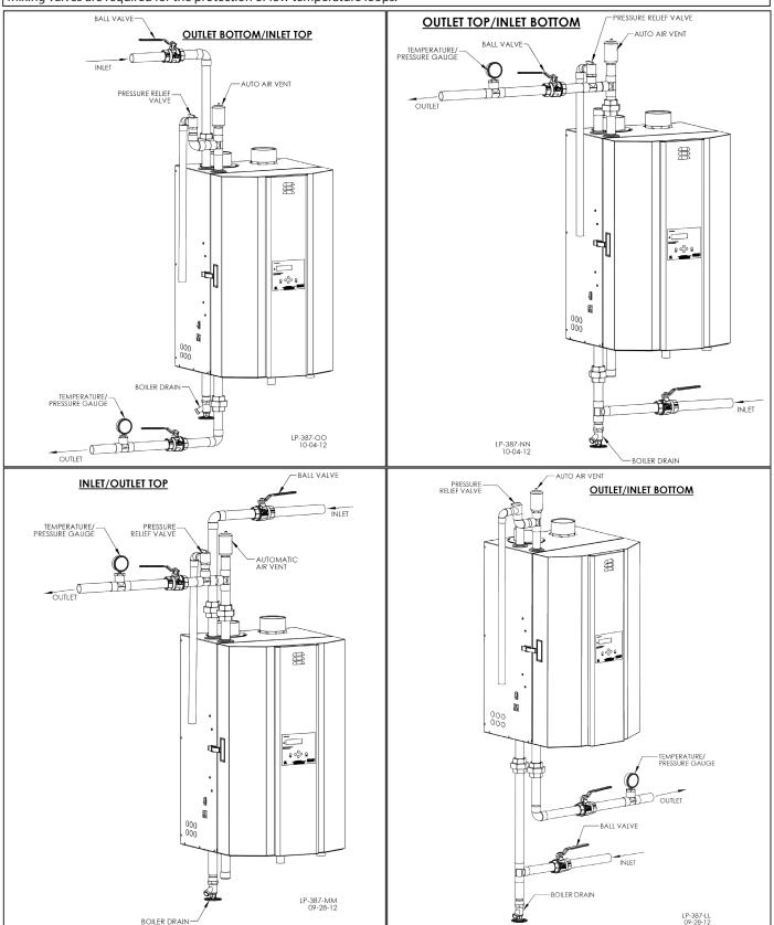
Figure 8 - Near Boiler Piping\* - NOTE: This drawing is meant to show system piping concept only. Installer is responsible for all equipment and detailing required by local codes. \*Top / Bottom Supply / Return Connections Available on 155 / 199 / 285 / and 399 Models ONLY.
