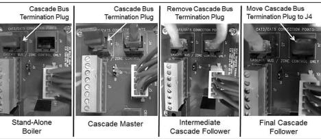
Figure 31 - Cascade Termination Plug Detail
