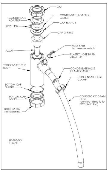
Figure 24 - Condensate Trap Detail
