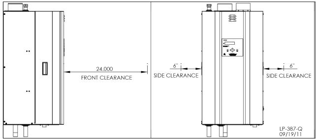
Figure 3 - Recommended Service Clearances
