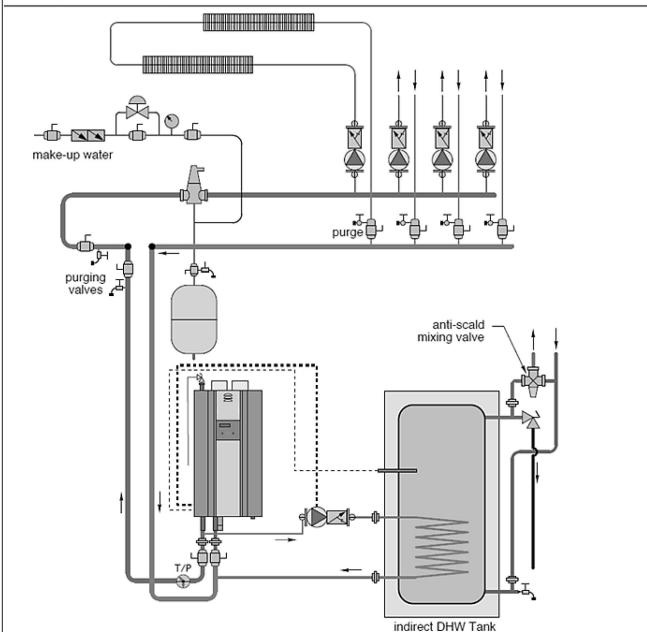
Figure 11 - Standard Piping with Pumps and Indirect Priority NOTES:
