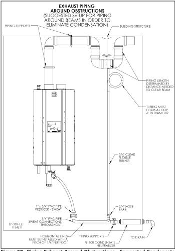
Figure 27 - Piping Exhaust Around Obstructions - Suggested Condensate Removal
