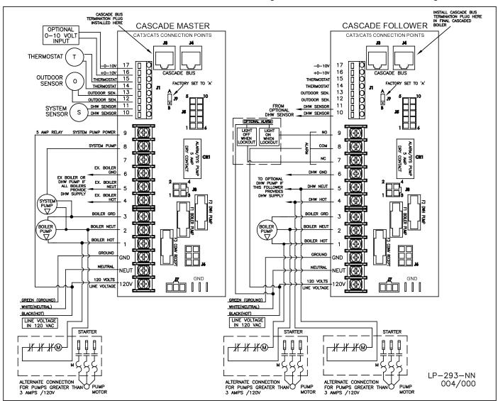
Figure 32 - Cascade Master and Follower Wiring
