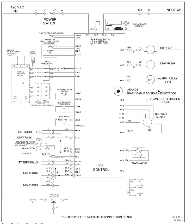
Figure 33 - Internal Connection Diagram
