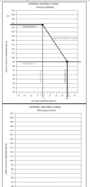
Table 23 - Heating Curve - NOTE: The user can adjust the heat curve down by lowering the central heating temperature.
