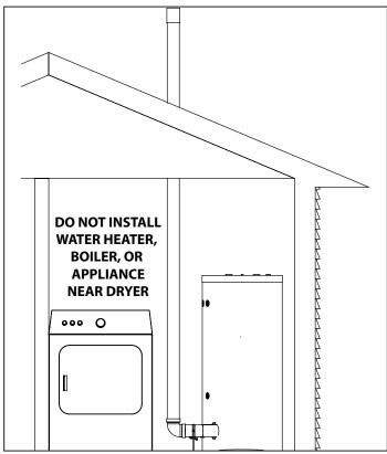
Figure 22 - Do Not Place Appliance Near Dryer
