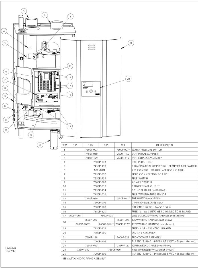
Figure 40 - Replacement Parts for all 155 and 199kBTU Models, and 285 - 399kBTU Models Manufactured BEFORE 10/29/17 - \*#15 - Switch on the Left is the Blocked Flue Pressure Switch on the Right is the Blocked Condensate Pressure Switch - Both share same Part Number
