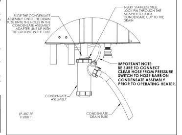
Figure 36 - Condensate Detail
