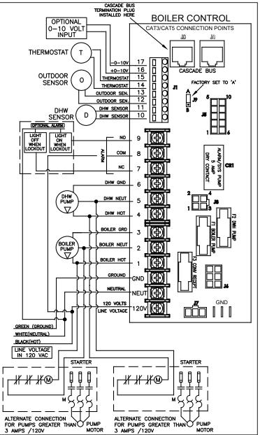
Figure 29 - Control Wiring
