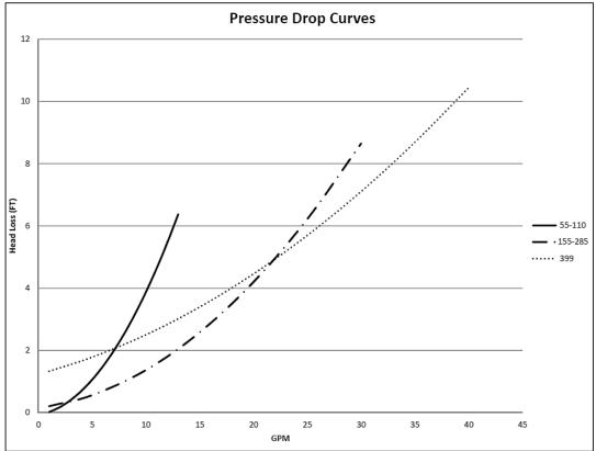
Figure 7 - Boiler Pressure Drop
