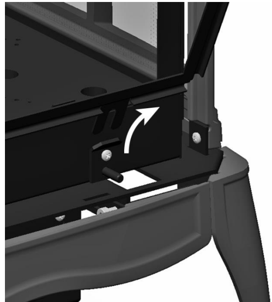
Figure 13 - Lower Mounting Stud/Spring Detail
