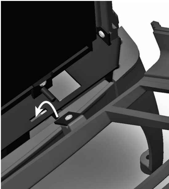
Figure 11 – Front Panel Retaining Slots
