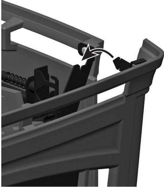
Figure 10 – Front Panel Mounting Tang Detail
