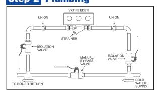
The feeder can be mounted on a horizontal or vertical cold water supply line. It must be installed with a manual by-pass valve and unions (as shown above) for future serviceability. Arrows on the valve indicate direction of water flow. Do not install feeder on hot water supply.
