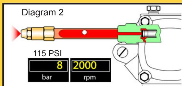
However, when the pump shuts down, it is a different story. As the pump's rpm decreases, the piston will close against the nozzle seat, cutting off the flow of oil from the pump, but not the flow of oil from the nozzle. The expanding bubble has taken over for the pump in supplying the pressure, pushing oil out of the nozzle. (diagram 2).
