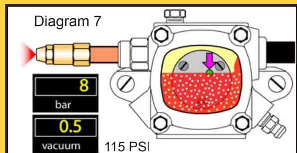
**The Tigerloop® prevents such air/gas problems by automatically and continuously de-aerating the oil before it enters the oil pump.**
