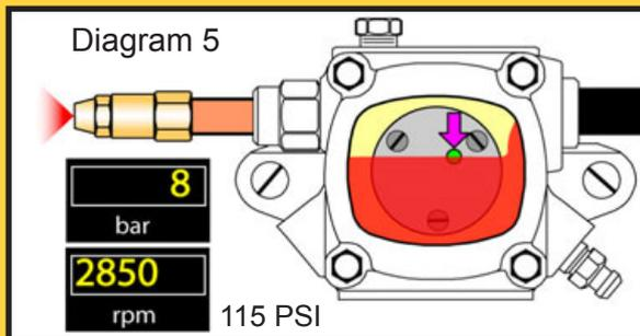
But, if air enters the pump, it will immediately rise to the top, pushing down the oil level in the strainer chamber and partially uncovering the inlet to the gear set. (diagram 5). The gear set starts gulping air and oil and the pressure becomes unstable, resulting in poor combustion, noise, rumbling, pulsation...
