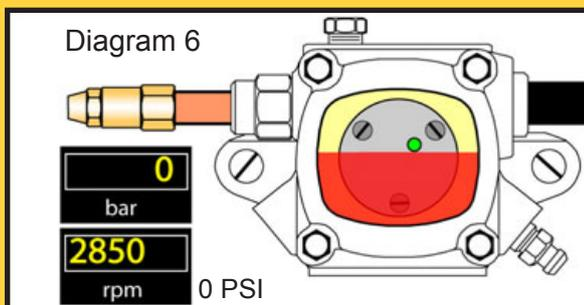
If enough air enters, the oil level drops completely below the inlet to the gear set, the pressure is lost and the burner eventually locks-out. (diagram 6).
