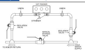
The feeder can be mounted on a horizontal or vertical cold water supply line. It must be installed with a manual by-pass valve and unions (as shown above) for future serviceability. Arrows on the valve indicate direction of water flow. Do not install feeder on hot water supply.
