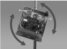
The VXT can be rotated to accommodate the orientation of the incoming water line. To rotate, loosen the 2 mounting screws located inside the housing (A) a quarter turn (these screws should NOT be removed from the housing). Rotate housing to desired position (clockwise or counter-clockwise). Once positioned, tighten the 2 mounting screws (A).
