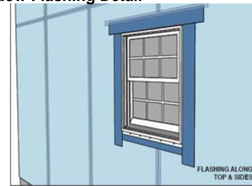
Figure 3 - Typical Window Flashing Detail
