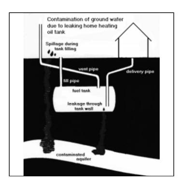
minimize the leaking potential of the tank or the piping connected to it. Even scratches in a metal tank caused by careless installation can increase corrosion and tank deterioration.
