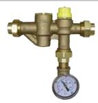
Apollo 34E Emergency Mixing Valves are designed to control the cold and hot water temperature to deliver tepid water at a predetermined temperature to emergency eyewash/facewash fixtures. The device provides a precise temperature and flow control in the event of cold water, hot water and thermostatic element failures. Complies with ANSI Z358.1-2009 & ASSE 1071-2008.
