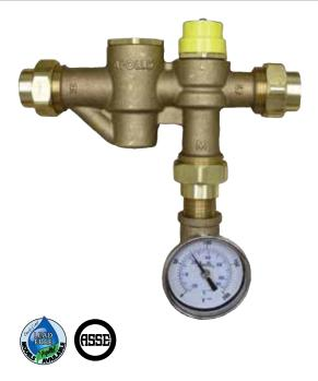
The Apollo® Model "MVE" (34E Series) emergency mixing valves are designed to control the cold and hot water temperature to deliver tepid water at a predetermined temperature to emergency eyewash/facewash fixtures. The device provides a precise temperature and flow control in the event of cold water, hot water and thermostatic element failures.
