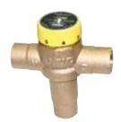
Apollo 34 Series mixing valves help extend hot water supply and enhance the life and accuracy of hydronic thermostats in residential and small commercial systems. These valves may be used to increase draw capacity of automatic storage water heaters. They save hot water and energy by automatically regulating the mix of hot water with cold. Water temperatures can be adjusted by simply turning the yellow knob to the desired setting.
