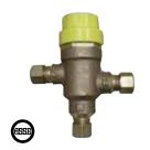
Apollo 34D Series thermostatic "Mini Mixer" valves are dual ASSE 1070 certified and designed as the ultimate single fixture valve, with a mixed accuracy of  $\pm$ - 2°F. Two designs are available depending on the application; single outlet design for sensor type faucets and double outlet design for standard connections.
