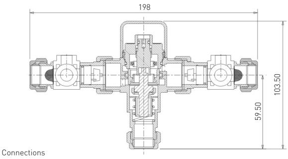
Inlet: 15mm compression Outlet: 15mm compression
