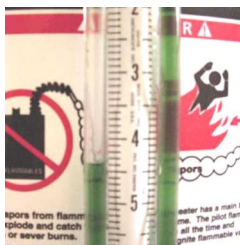
Common Testing Device use for a Leak Test
