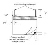
Figure 15-22: Hand seal caps as shown.
