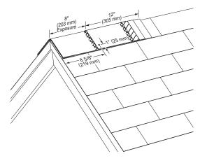
Figure 15-21: Install cap shingles at an 8" exposure and fasten with one nail on each side as shown.
