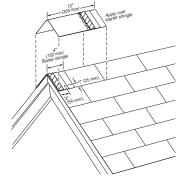
Figure 15-20: Apply a full cap shingle over the starter shingle.
