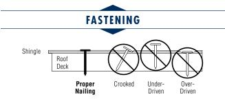
Figure 15-5: Proper and improper nailing.
