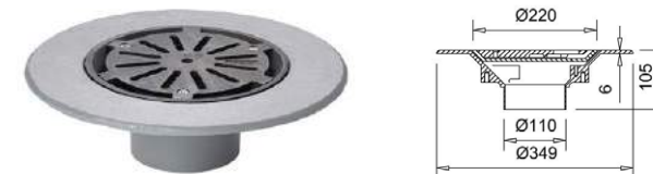
Frost floor drain 200mm circular flat grating with medium sump body and spigot outlet
