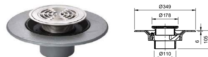
Frost floor drain 178mm circular grating for vinyl floors with medium sump body and spigot outlet
