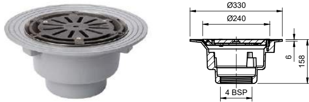
Frost floor drain 240mm circular flat grating with large sump body and threaded outlet
