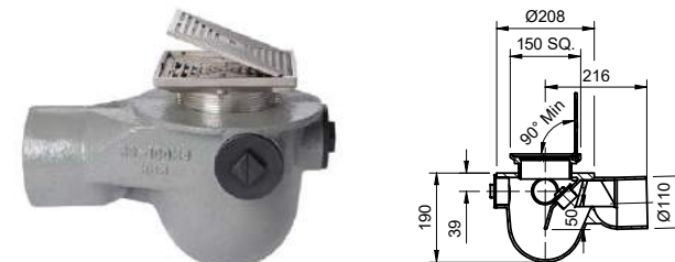
Frost floor drain 150mm square grating with hinged cover plate with medium sump – 'P' trap – spigot outlet
