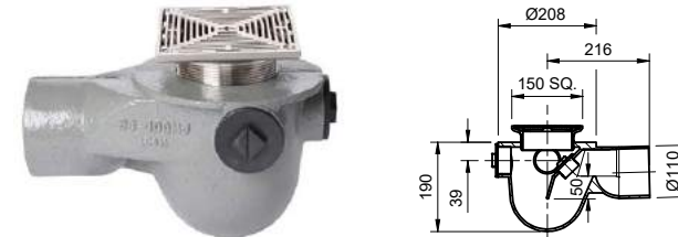
Frost floor drain 150mm Slimline Heel Proof slotted grating with medium sump – 'P' trap – spigot outlet
