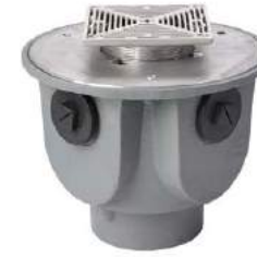
Frost floor drain 150mm Slimline Heel Proof slotted grating with large deep sump body and threaded outlet
