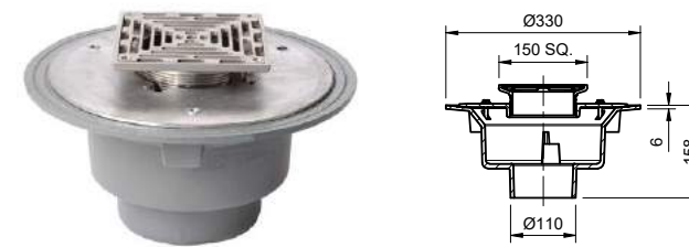
Frost floor drain 150mm square grating with large sump body and spigot outlet
