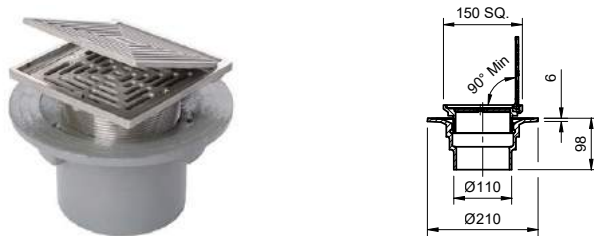
Frost floor drain 150mm square grating with hinged cover plate with small sump body and spigot outlet
