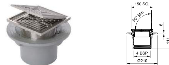
Frost floor drain 150mm square grating with hinged cover plate with small sump body and threaded outlet
