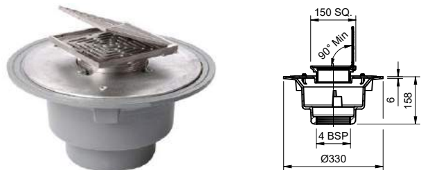
Frost floor drain 150mm square grating with hinged cover plate with large sump body and threaded outlet
