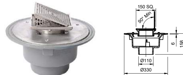
Frost floor drain 150mm square grating with hinged cover plate with large sump body and spigot outlet
