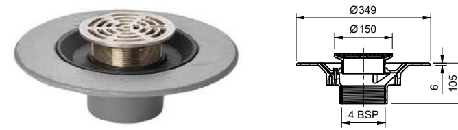
Frost floor drain 150mm circular grating with medium sump body and threaded outlet
