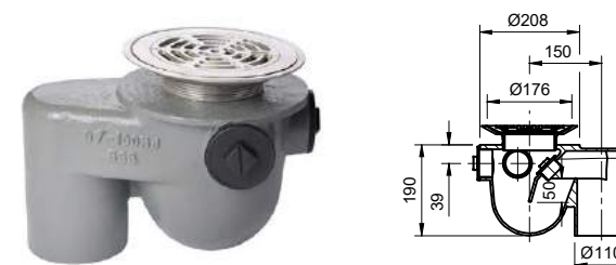
Frost floor drain 178mm circular grating for vinyl floors with medium sump – 'S' trap – spigot outlet
