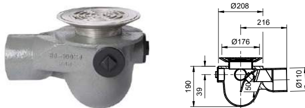
Frost floor drain 178mm circular grating for vinyl floors with medium sump – 'P' trap – spigot outlet
