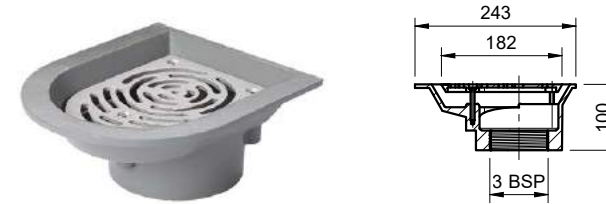
Frost balcony outlet aluminium grating with small sump body and threaded outlet
