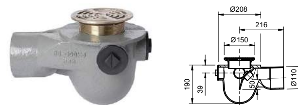
Frost floor drain 150mm circular grating with medium sump – 'P' trap – spigot outlet
