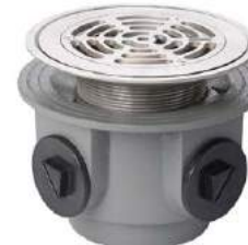
Frost floor drain 178mm circular grating for vinyl floors and medium sump body with side inlets and threaded outlet
