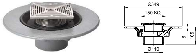
Frost floor drain 150mm Slimline Heel Proof slotted grating with medium sump body and spigot outlet
