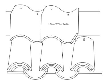
11. Install the 1-Piece "S" Tile or Claylite<sup>®</sup> tile directly over the top edge of the 2-Piece Mission eave treatment. Ensure that a minimum 3" headlap is maintained.
