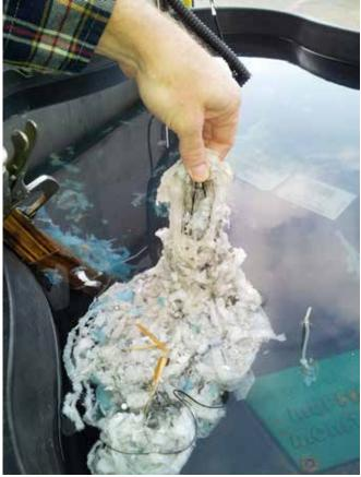
Rag balls form in collections systems when debris and hair knit together. Research revealed that hair is the main catalyst for the rag balls. JWC Environmental
