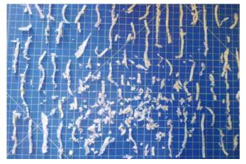
developed that includes ultrahigh molecular weight (UHMW) plastic screening panels. This new system not only allows the screen panels to withstand the harsh environment, but also prevents debris from "stapling" or getting stuck to the panels. Stringy debris can get caught when the two ends are pushed into two adjacent perforated holes at the same time. The debris has become "stapled" to the panel, similar to the way a staple goes through a piece of paper and gets locked in.
