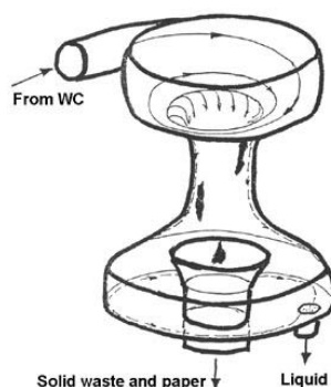
Figure 15: The Aquatron (Vinneras and Jonsson 2002)
