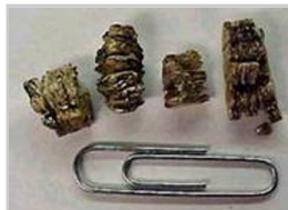
Vermiculite insulation particle size relative to paper clip; click to view larger version of image
