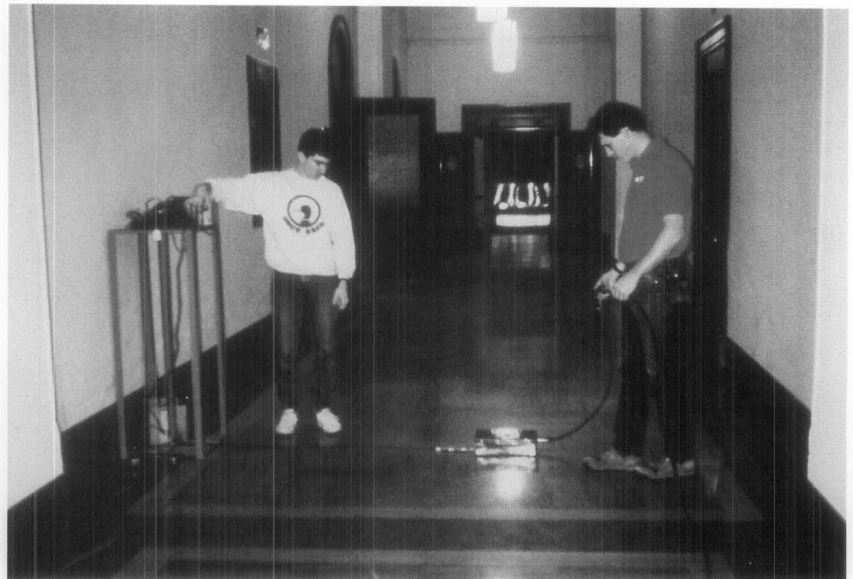
Figure 2. (a) The floor structure is scanned using impulse radar. An operator is shown, pushing the transducer across the floor surface at a constant speed. (b) The transducer is being pulled, by machine, at a constant speed. Photos: Marie Ennis, P.E.
