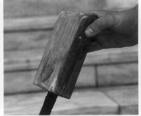
Fig. 12. (left) Raw radar output was analyzed by the geophysicists. Correlations could then be made to provide qualitative and quantitative evaluations of the stone. (right) This impulse radar transducer emits and receives electromagnetic energy. The unit is attached directly to the equipment shown at left. Photos: Edmund P. Meade, P.E.
