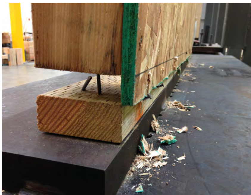
Fastener tearing through sheathing
