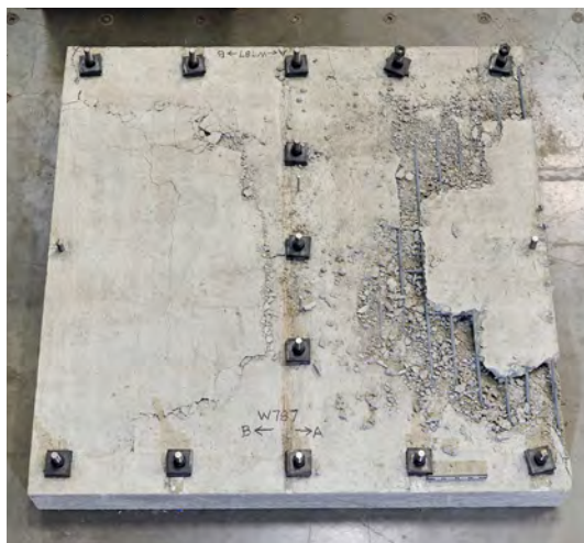
Anchor reinforcement testing at Tye Gilb Laboratory for edge and away-from-edge conditions.
