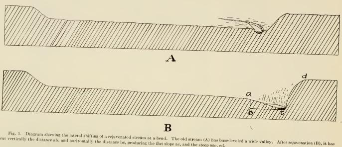
cut vertically the distance ab, and horizontally the distance bc, producing the flat slope ac, and the steep one, ed.
