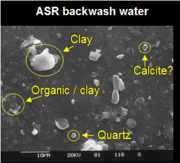
Figure 9. SEM micrographs showing particles in backwash water from ASR well on 10 Dec. 1999
