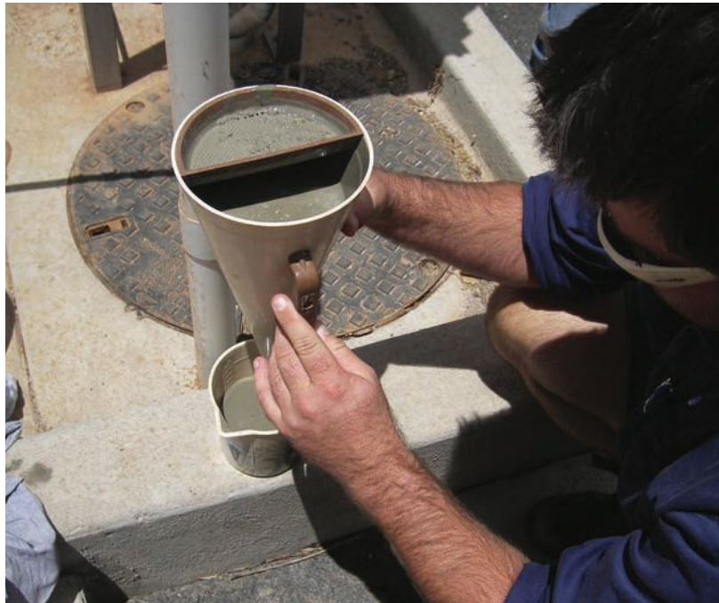
Measuring viscosity using a Marsh funnel
