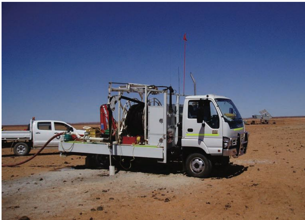
Mobile pump test unit (small flow)
