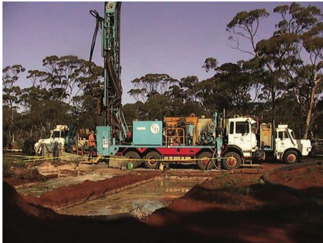
Rotary mud drilling
