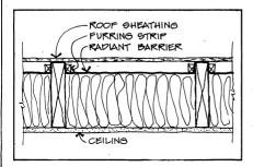
A. The foil is in the right place to block radiant heat across the airspace. But there are some other problems. First, radiant barriers are not really cost effective in cold climates such as yours. Their primary use is to reduce cooling loads in hot climates. Second, in winter a continuous layer of foil above the insulation creates a cold-side vapor barrier, vulnerable to condensation on the underside.
