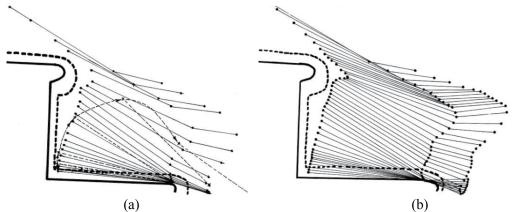
Figure 5. Analyses, from video, of two descents of a mocked up home stair, both showing interactions of step geometry and descent gait of one shod foot, with back of shoe heel, ball of the foot and front of the shoe sole indicated in two-segment lines each 1/24 second apart
