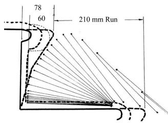
Figure 6. Analysis of foot pivot on lift off from a home stair tread as a basis for a redesign of the interface of the nosing and closed riser, preferably with a compound back slope
