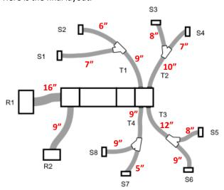
Note that some of the t-wyes are incorrectly drawn. Usually, the larger duct is in-line with the trunk, and the smaller duct branches off at an angle. The drawing can be fine-tuned after you determine the duct sizes. Different style fittings can also be used depending on your preference (duct board boxes, pants, etc.).
