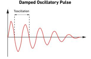
equipment is planned to operate. The frequencies for common IEC oscillatory pulses span from 100 kHz to 30 MHz including all three categories.
