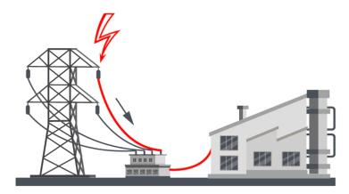
Transients can be transmitted down electrical paths from device to device having the potential to impact a large amount of electrical equipment. Given the wide number of potential culprits, waveforms used to characterize these events also can vary widely based upon the application and anticipated environment.
