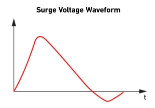
When evaluating rise times of impulse transients, it is common to see that waveforms with faster rise times have a shorter duration. Compare the pulse above 1.2us by 50us to an electrical fast transient pulse (IEC 61000-4-4) which is 5ns by 50ns.
