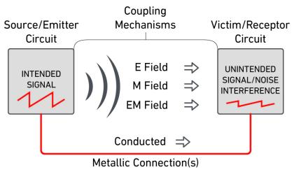
There are three basic noise mechanisms for coupling transient noise into target electrical systems/subsystems/printed circuit board or board traces.
