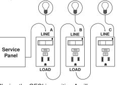
Placing the GFCI in position A will also provide protection to "load side" receptacles B and C. On the other hand, placing the GFCI in position C will not provide protection to receptacles A or B. Remember that receptacles A, B, and C can be in different rooms.
