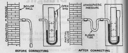
FIGS. 2 and 3-U type draught gauge, at zero before connecting, and indicating 2 inches after connection. In reading, since the column in the two tubes fall and rise equal distances, take the reading of one leg only and double it to obtain the draught in inches.
