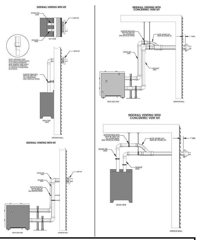
NOTE: When placing support brackets on vent piping, the first bracket must be within 1 foot of the appliance and the balance at 4 foot invervals on the vent pipe. The boiler venting must be readily accessible for visual inspection for the first three feet from the boiler.
