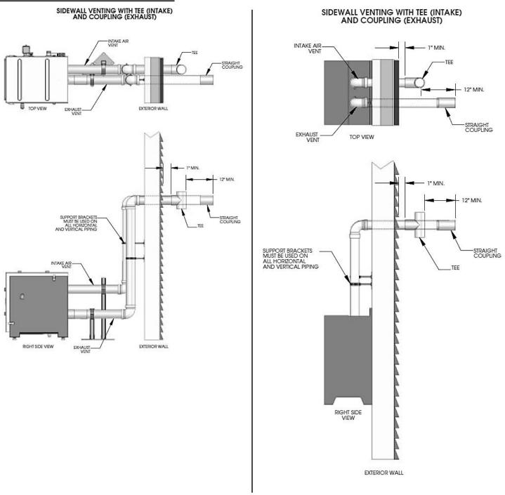
GENERAL NOTE: All vent pipes must be glued, properly supported and the exhaust must be pitched a minimum of a 1/4" per foot back to the heater (to allow drainage of condensate).
