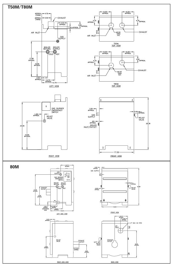
Figure 1 - Dimensions - T-50M / T-80M / 80M
