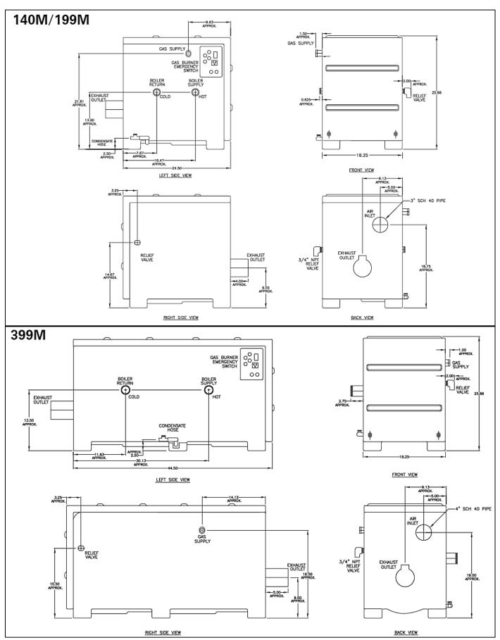
Figure 2 - Dimensions - 140M / 199M / 399M
