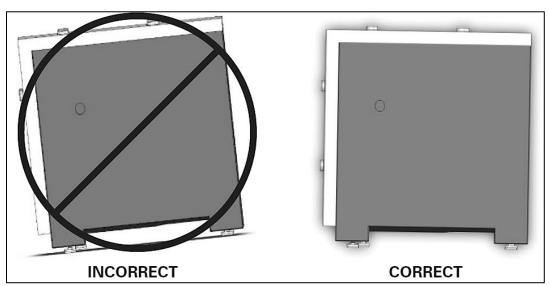
Figure 3 - Boiler Leveling
