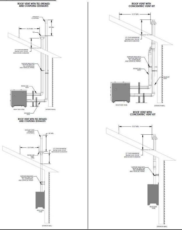
NOTE: When placing support brackets on vent piping, the first bracket must be within 1 foot of the appliance and the balance at 4 foot invervals on the vent pipe. The boiler venting must be readily accessible for visual inspection for the first three feet from the boiler.
