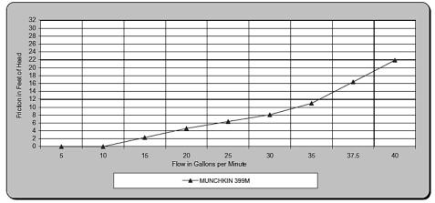
\* NOTE: The recommended circulators are based on 1 gpm per 10,000 btu/hr with 20°∆t.
