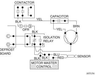
Fig. 3 - 460-v Wiring for Motor Master
