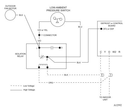
Fig. 1 - Wiring for Low-Ambient Pressure Switch
