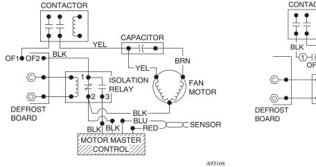
Fig. 2 - 208/230-v Wiring for Motor Master
