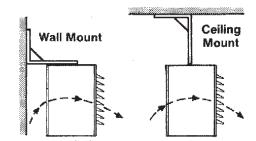
Attach heater to bracket with 3/8" x 1" bolt & lock washer supplied with bracket. After desired air discharge position has been determined, tighten bolt so the heater will not pivot.
