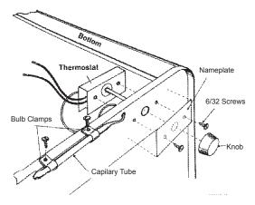
**Stainless Steel Models** require a special thermostat model (TF115) that will be mounted to the outside of the heater. This must be sealed properly and is recommended to be done at the manufacturing plant. For additional information please consult the factory.
