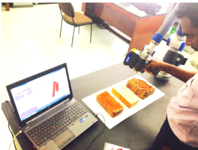
Fig. 3. Studying surface roughness by using 3d scanner.
